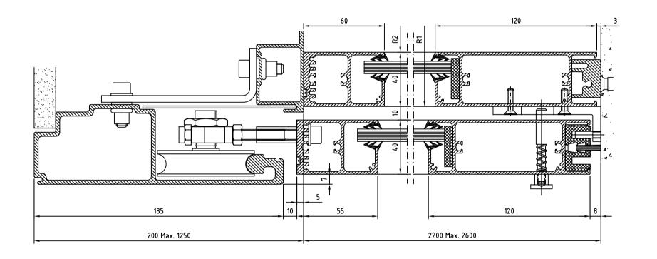
Revolving door **RD3/4 Frame NCD** Section NCD Standard fascia
