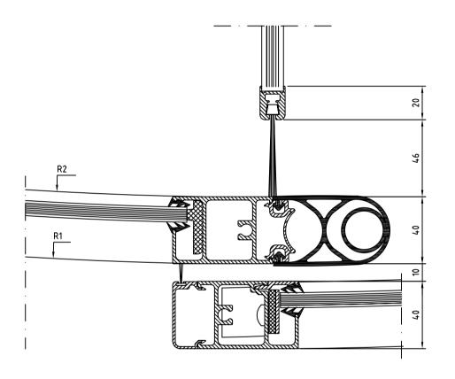
Revolving door RD3/4 Frame wall - Slim doorleaf NCD Section door-wall
