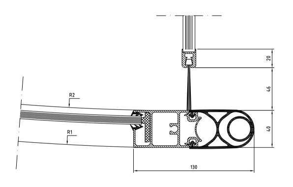
Revolving door RD3/4 Frame wall - Slim doorleaf Section Door - wall
