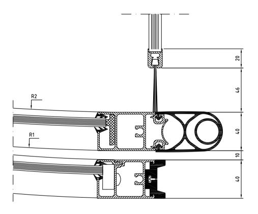
Revolving door RD3/4 Frame wall - Slim dorrleaf NCD Section door - wall
