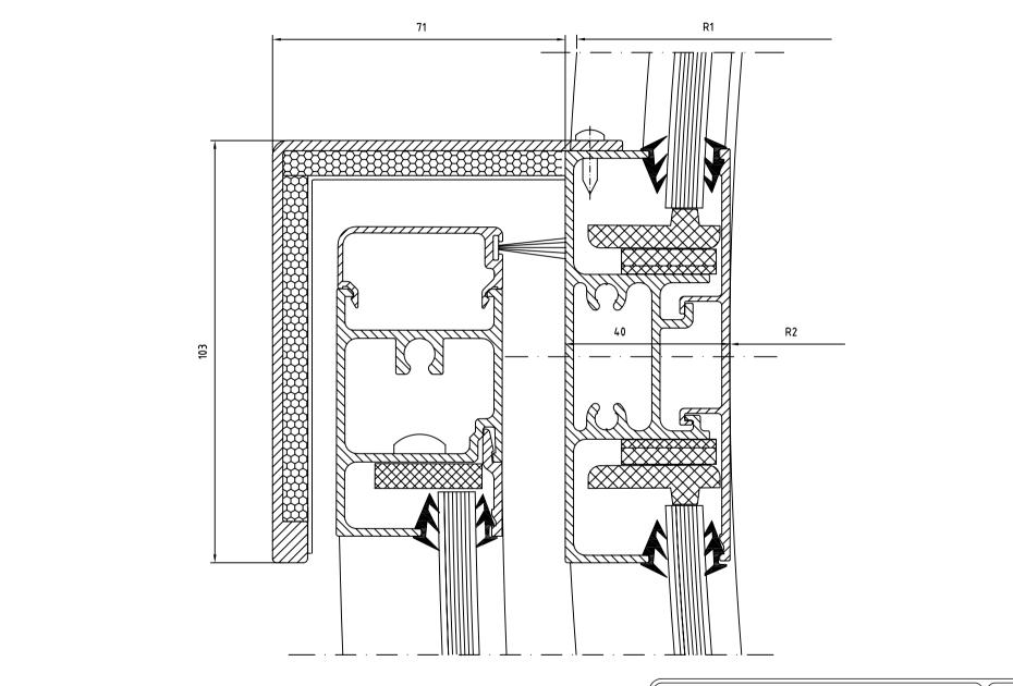
Revolving door RD3/4 Frame NCD Section NCD slam post
