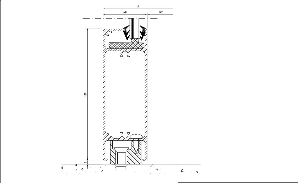
Revolving door RD3/4 Frame Section Bottom - outer wall
