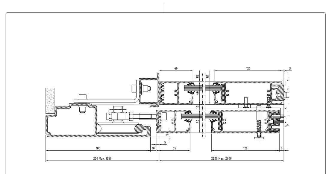
Revolving door RD3/4 Frame NCD Section NCD Standard fascia
